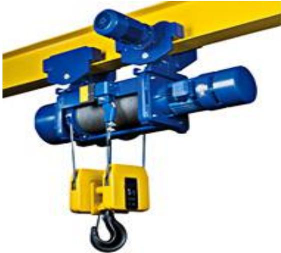
Standard headroom monorail design enables the hoist to operate directly under and parallel with the crane or runway beam. The hoist is suspended via drive trolley. Application in single girder cranes where space is not an issue.
