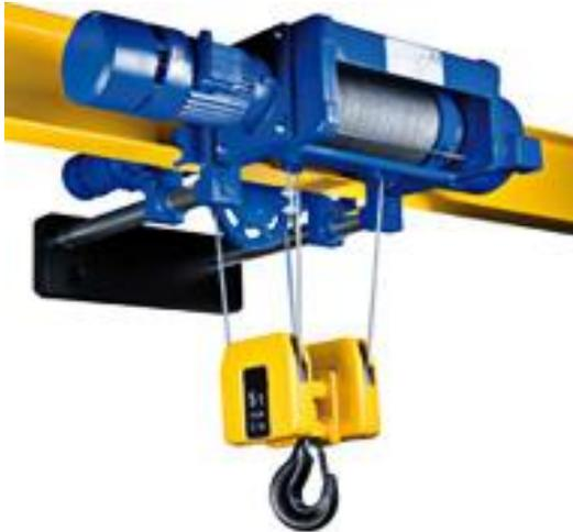
The low room headroom trolley consists of two electric trolley motors with planetary gearbox. The trolley is of a live axel design with the gearboxes fitting directly onto the drive shaft of the wheels removing the need of external gears. Most common solution for single girder cranes. Compact design for maximum space utilization.
